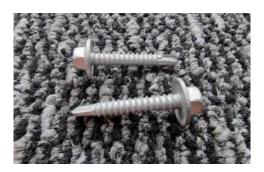
Screw Type:Steel-Fast Self Drilling (SD) – 12-14 x 35mm longHead Type:Hexagon HeadHead Markings:SX3Head (Nominal):7.8mm Across Flats (A/F) – To suit 5/16" driverCoating Type:Sure-guard 3
