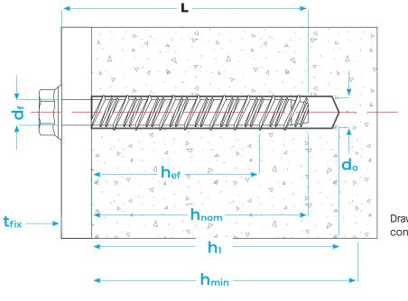
Drawing A1. Installed condition for screw-bolt
