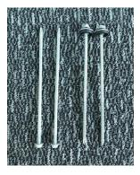
Screw Type 1:Timber Self Drilling (SD) – Type 17 14-10 x 200mm longHead Type:Hexagon HeadHead Markings:SX4Head (Nominal):9.4mm Across Flats (A/F) – To suit 3/8" driverCoating Type:Zinc
