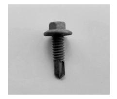
Screw Type 1:Sure-Fast Shed-Fast Self Drilling (SD) – 14 x 22mm longHead Type:Hexagon Washer HeadHead Markings:SX3Head (Nominal):7.8mm Across Flats (A/F) – To suit 5/16" driverCoating Type:Zinc
