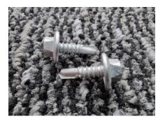
Screw Type:Steel-Fast Self Drilling (SD) – 12-14 x 20mm longHead Type:Hexagon HeadHead Markings:SX4Head (Nominal):7.8mm Across Flats (A/F) – To suit 5/16" driverCoating Type:Sure-guard 3
